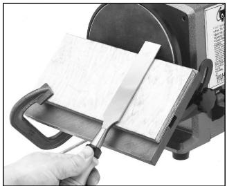
Figure 11. Auxiliary table for sharpening.
